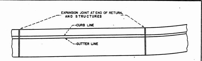
0.0495 CUBIC YARDS PER LINEAL FOOT. 20.2 LINEAL FEET PER CUBIC YARD. Survey reference point (#10 Round Head Brass Screw, minimum length 1 1/4") set flush at end of curb return during construction. CURB **CURB LINE** ELEVATION-PLACE PAVEMENT 1/4" ABOVE CONCRETE 1/2"R. i/2"R -!/2"R ~ | 1/2" 4 PREMOLDED EXPANSION JOINT FILLER 1/4"-/PERMITTED 24" ALTERNATE SECTION **EXPANSION JOINT**
