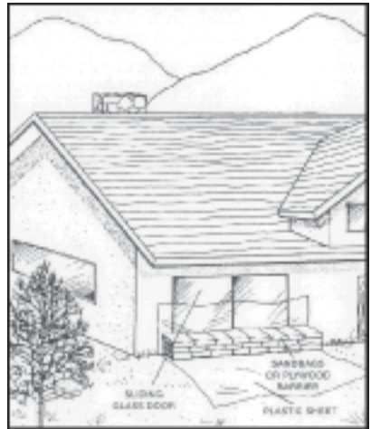
Sliding glass door sealing.
