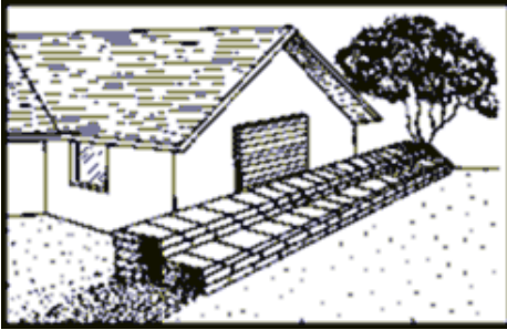
Sandbag stacking against buildings.
